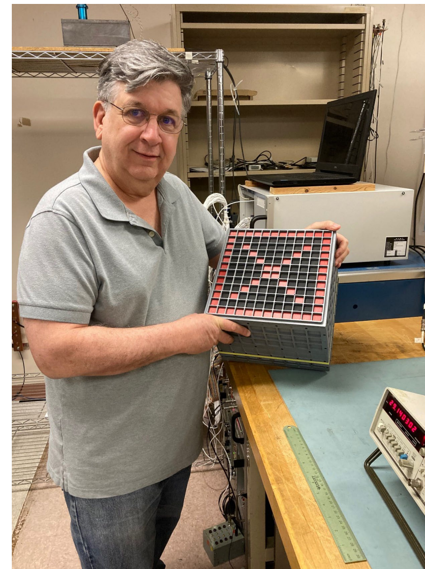
A 3d-printed full-scale model of one LEAP Polarimeter Module.
